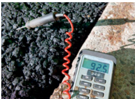
Asphalt is produced at temperatures of just below 100°C, reducing carbon emissions and fuel consumption by up to 50%
